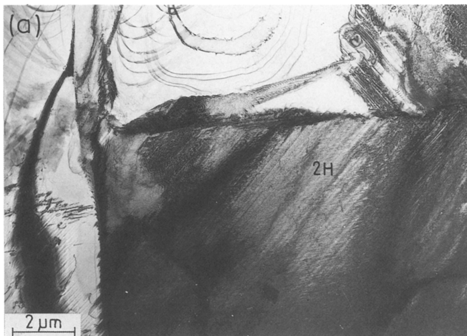
Figure 4 Set of transmission electron micrographs taken with decreasing strain (see Fig. 1) corresponding to decreasing of the 2H martensite area: (a) electron diffraction pattern from the \beta_1 area are shown in (c).
