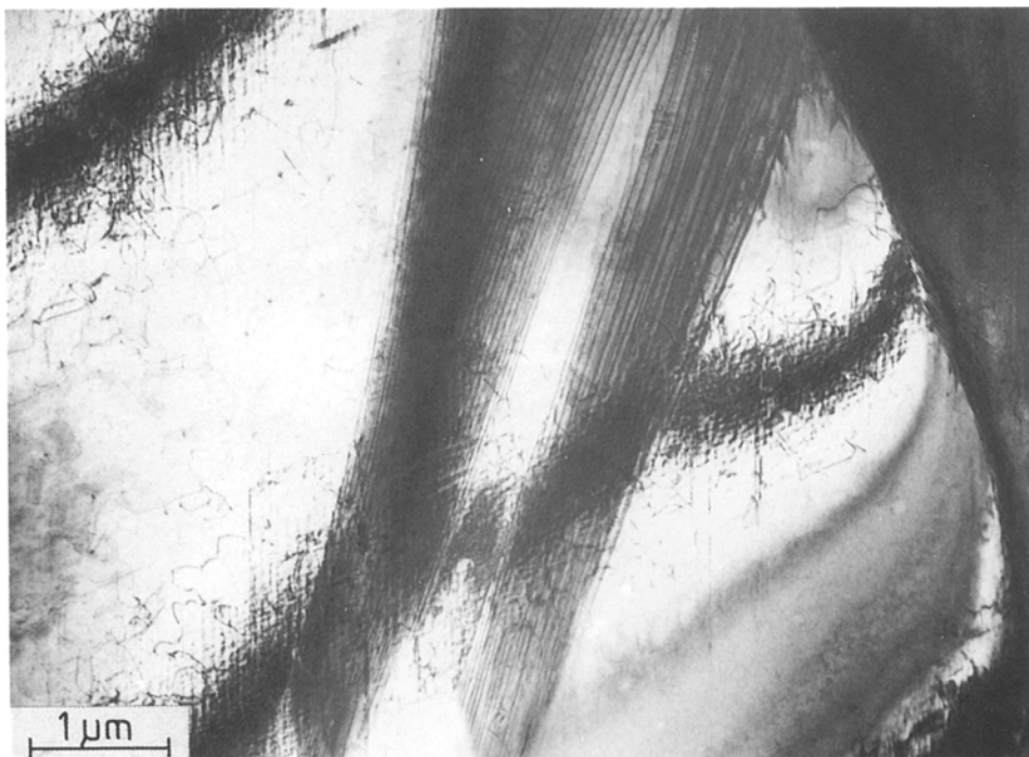
Figure 10 Transmission electron micrograph taken during strain release in the second cycle showing two variants of martensite.
